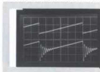
Top waveform is 100Hz Sawtooth input. Bottom is VCF output at 1KHz Cutoff Q=5
