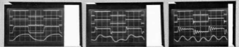
Top waveform in all 3 pictures displays 300-Hz Square wave input. Next wave is VCF output at 16 kHz cutoff. Next wave is VCF output at 10 kHz cutoff. Bottom wave is VCF output at 250-Hz cutoff. Picture at left Q = 0.5, Center Q = 2, Right Q = 5.
